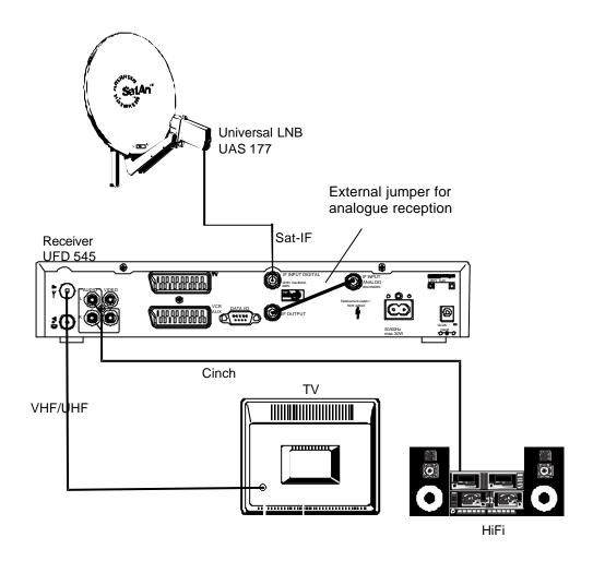
Connection of a TV set without a SCART socket to the modulator output of the receiver. The signal is looped through via the video recorder to facilitate VCR operation.
